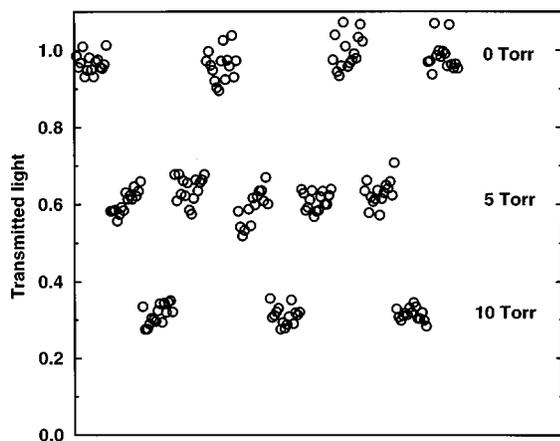
FIG. 3. Transmission through the absorption cell for three different pressures of CO and excitation on the  $Q_2(2)$  line. The first 15 data points are recorded with an evacuated cell. For the next 15 data points the cell is filled with 5 Torr of CO, after that with 10 Torr of CO, etc. The vertical axis is adjusted to a transmittance of unity for an evacuated cell.
