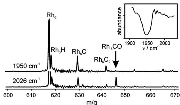
**Figure 1.** Mass spectra in the region of  $\text{Rh}_6$  with FELIX on ( $1950\text{ cm}^{-1}$ ) and off ( $2026\text{ cm}^{-1}$ ) the  $\nu(\text{CO})$  resonance in the  $\text{Rh}_6\text{CO}$  complex. Inset shows the frequency dependence of the  $\text{Rh}_6\text{CO}$  signal.
