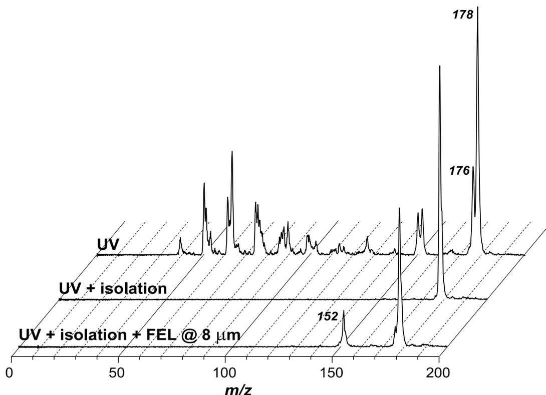
Fig. 2.—Mass spectra of cationic phenanthrene in the experimental sequence used in the IR MPD technique
