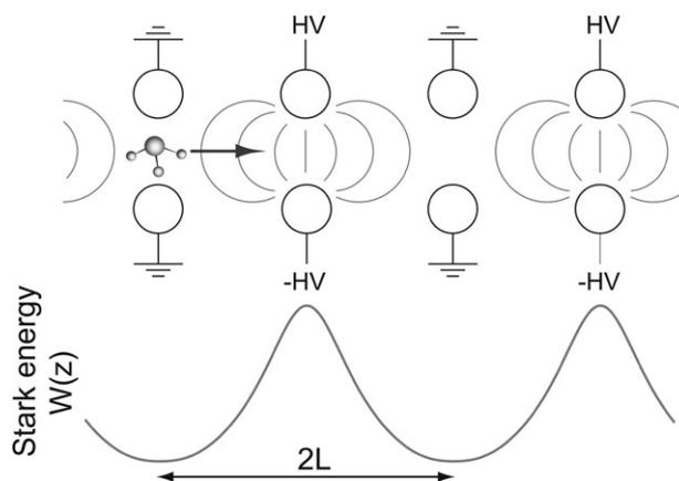
**Fig. 1** Scheme of the Stark decelerator. The Stark energy of a  $\text{ND}_3$  molecule in a low-field seeking quantum state is shown as a function of position  $z$  along the molecular beam axis. The Stark energy has a period of  $2L$ .
