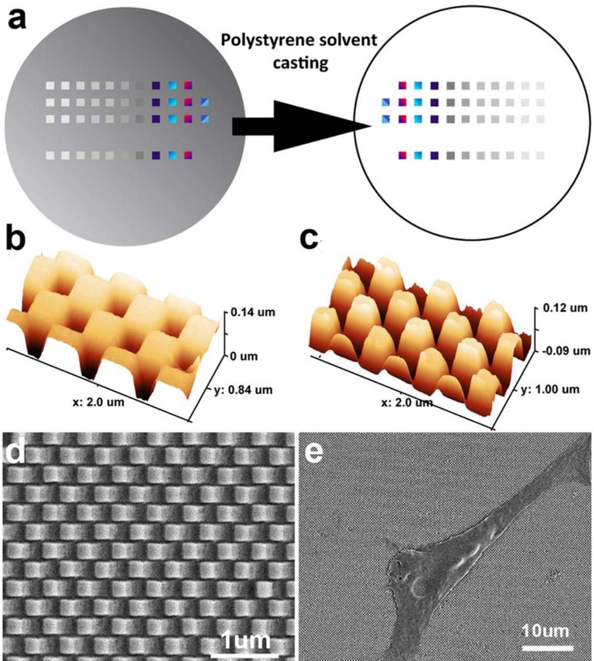
**Fig. 2.** Polystyrene Biochips are produced from a silicon template and used for biological analyses. **a.** Using polystyrene solvent casting replicas were created containing 40 different field patterns. The **b.** silicon mould and **c, d.** polystyrene replicas were routinely checked with AFM and high resolution SEM. **e.** Polystyrene replicas were finally used for biological analyses.
