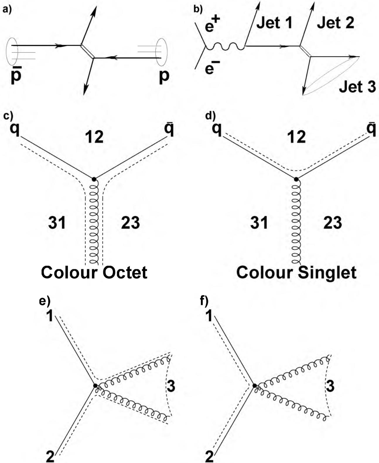
Figure 1: Schematic diagram of colour exchange. Colour singlet propagators are indicated by double lines in a)  $p\bar{p}$  and in b)  $e^+e^-$  reactions. The  $e^+e^-$  diagram is derived by crossing the incoming quark line in the  $p\bar{p}$  diagram. Colour flow is shown by dashed lines for c) COP and d) CSP in 3-jet events from  $e^+e^-$  annihilation and also e) without and f) with colour reconnection.
