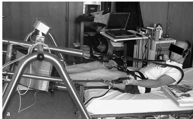
Fig. 1a “Galileo Space” training device for usage in bed-rest. The subjects attach themselves to a vibrating platform by belts with their waist, their shoulders, and their hands. Vibration is generated by means of eccentrically rotating masses on the other (= left) side of the platform.
