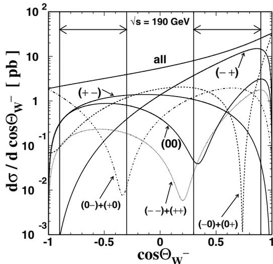
**Fig. 1.** Differential cross section for pair production of polarised W bosons at  $\sqrt{s} = 190$  GeV averaged over initial electron polarisations. The  $W^-$  and  $W^+$  helicities in the  $e^+e^-$  centre-of-mass frame are given in parentheses. The intervals used for the analysis of W-boson spin correlations are indicated by the arrows
