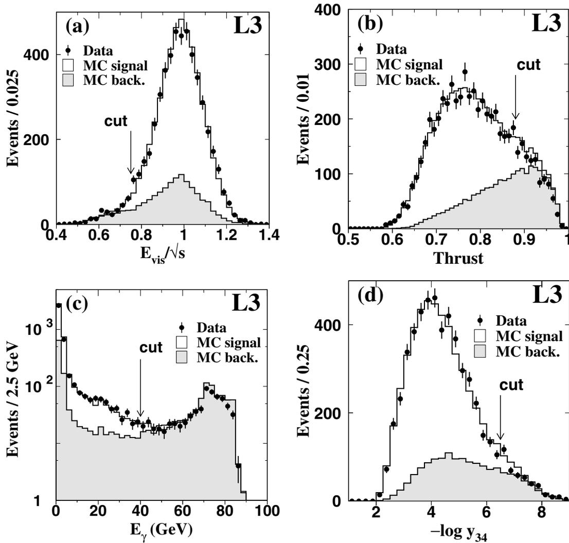
**Fig. 3.** Distributions of variables used for the selection of  $e^+e^- \rightarrow W^+W^- \rightarrow q\bar{q}q\bar{q}$  events: **a** normalised visible energy, **b** event thrust, **c** energy of the most energetic photon,  $E_\gamma$ , **d** jet-resolution parameter,  $-\log y_{34}$ . In each plot, all other selection criteria are applied. The arrows indicate the positions of the cuts
