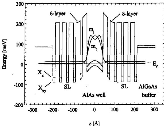
Fig. 1. Diagram showing the potential energy at the X minimum of our modulation-doped AlAs QW structure. The wave-functions and potential are shown for a 2DEG with an electron density of  $1.5 \times 10^{12} \text{ cm}^{-2}$ . The splitting of the X-band is indicated for the SL and the AlAs well. The energy is measured with respect to the energy at the centre of the well, when no strain is included.
