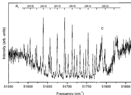
Fig. 6. Spectrum of the  $D \ ^2\Sigma^+(\nu' = 0) \leftarrow X \ ^2\Pi(\nu'' = 1)$  transition of NO measured with the remaining 193-nm ( $F_{00}$ ) radiation behind the Raman cell. Identification of the strongest lines,  $R_{11}$  branch, is indicated.
