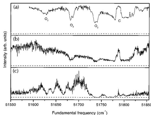
Fig. 4. Intensity profiles of (a) the 193-nm radiation of the excimer laser, (b) the remaining 193-nm radiation behind the cell ( $F_{00}$ ), and (c) the generated 224-nm radiation ( $F_{11}$ ) shifted by 7142.3  $\text{cm}^{-1}$ . Zero intensities are indicated by dashed lines.
