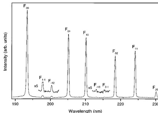
Fig. 2. Stimulated Raman scattering of ArF excimer laser radiation (at 193.4 nm) in a mixture of 19%  $\text{H}_2$  in  $\text{D}_2$  at a total pressure of 25 bars. The designation of the lines is explained in the text. The figure is not corrected for any wavelength-dependent detection efficiency.
