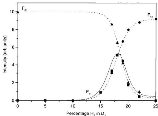
Fig. 3. Relative intensities of the first Stokes lines of  $\text{H}_2$  ( $\bullet$ ,  $F_{10}$ ),  $\text{D}_2$  ( $\blacktriangle$ ,  $F_{01}$ ), and the 224-nm line ( $\blacksquare$ ,  $F_{11}$ ), as a function of the percentage of  $\text{H}_2$  in  $\text{D}_2$  (total pressure 25 bars).
