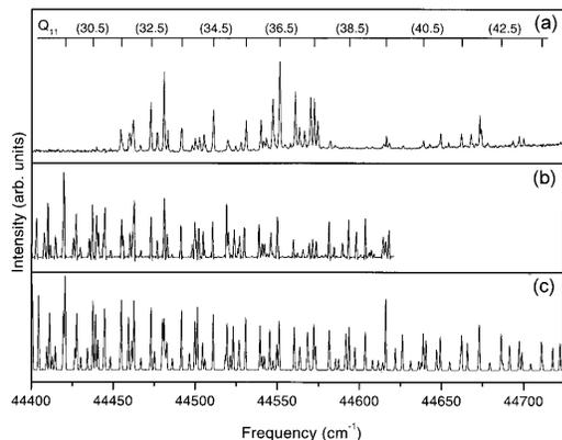
Fig. 5. Spectra of the  $A \ ^2\Sigma^+(\nu' = 0) \leftarrow X \ ^2\Pi(\nu'' = 0)$  transition of NO (a) measured with the 224-nm radiation ( $F_{11}$ ) generated in the Raman cell, (b) measured with a frequency-doubled dye laser, and (c) simulated with data from Reisel *et al.*<sup>13</sup> Identification of the  $Q_{11}$  branch is indicated.
