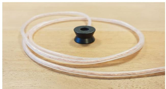
**FIGURE 2** Suction device to measure skin elasticity, DermaLab Combo® [Colour figure can be viewed at [wileyonlinelibrary.com](http://wileyonlinelibrary.com)]
