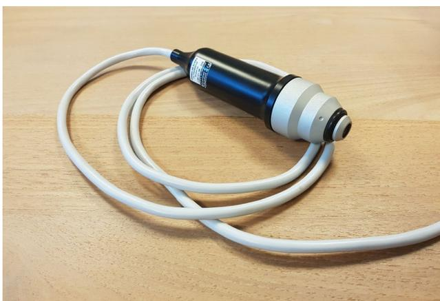
**FIGURE 1** 20-MHz echoprobe to measure skin thickness, DermaLab Combo® [Colour figure can be viewed at [wileyonlinelibrary.com](http://wileyonlinelibrary.com)]
