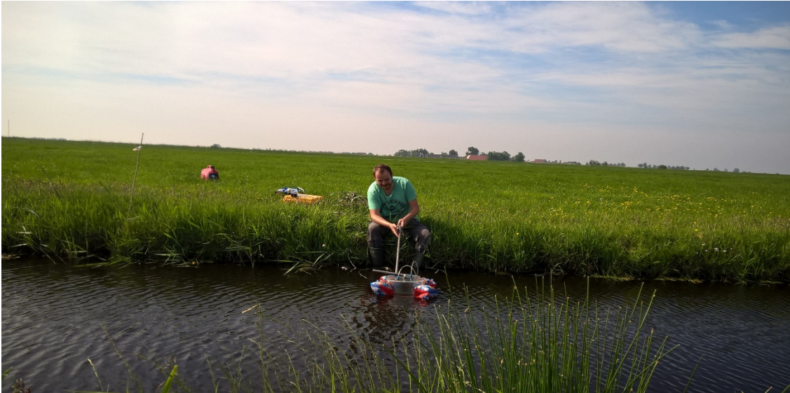
Diffusive flux measurements with floating chamber and Los Gatos (left) and bubble traps for ebullitive flux measurements (right)
