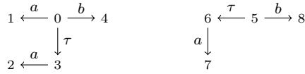
Figure 3: An illustration of the difference between weak bisimulation and branching bisimulation: states 0 and 5 are weak bisimilar but not branching bisimilar.
