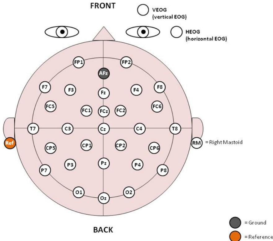
**Figure 2. Schematic of electrode placement based on the international 10-20 system.** The white electrodes represent the applied placement of the 32 active electrodes with linked mastoid reference placement and two active electrodes used for EOG measurement. The orange electrode represents the reference electrode. The gray electrode represents the ground electrode. [Please click here to view a larger version of this figure.](#)
