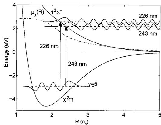
FIG. 3. Photodissociation of OD  $X^2\Pi(v=5)$  at 226 and 243 nm via the repulsive  $1^2\Sigma^-$  curve depicted with *ab initio* potentials, bound state and continuum wave functions, and transition dipole moment function (arbitrary units). The photodissociation cross section is large at 243 nm, but poor overlap of the wave functions when starting from  $v=5$  results in minimal products at 226 nm, as seen experimentally.
