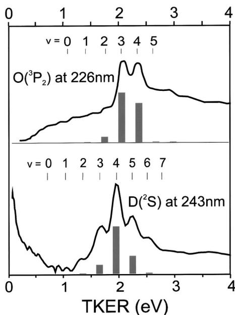
FIG. 2. Total kinetic energy release (TKER) derived from velocity map images of  $O(^3P_2)$  and  $D(^2S)$  fragment atoms following photodissociation of OD at 226 and 243 nm, respectively. The initial vibrational state of OD is determined from energy balance with  $TKER = h\nu + E(\text{vib})_{OD} - D_0$ . The bar graphs show the calculated photodissociation yields for OD  $X^2\Pi(v)$  at a vibrational temperature of 1700 K.
