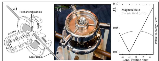
**Fig. 2.** Schematic drawing (a) and photograph (b) of the permanent magnetic trap. In (c) the loading potential and the trapping potential for NH ( $a^1\Delta(v=0, J=2)$ ) radicals is shown with respect to the midpoint between the two disc-shaped electrodes.
