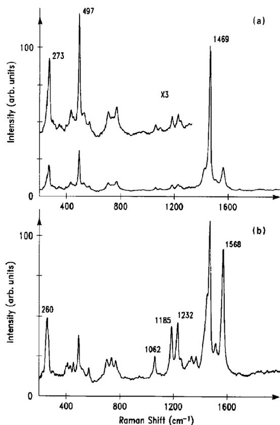
Fig. 2. Unpolarized Raman spectra of purified films of  $C_{60}$  and  $C_{70}$  on suprasil substrates with a and b corresponding to mass spectra a and b shown in fig. 1. The labelled lines in spectra a and b are assigned to  $C_{60}$  and  $C_{70}$ , respectively. In both spectra the intensity of the line at  $1469\text{ cm}^{-1}$  is normalized to 100.
