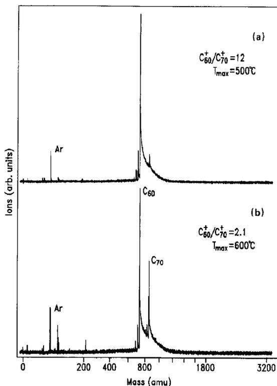
Fig. 1. Time-of-flight mass-spectra of purified films of  $C_{60}$  and  $C_{70}$  on tungsten foil, taken using the laser-desorption jet-cooling mass spectrometer. The horizontal axis is linear in time-of-flight and the corresponding (nonlinear) mass scale is indicated. The maximum sublimation cell temperatures,  $T_{\max}$  are indicated.
