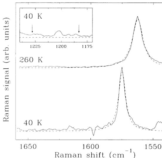
FIG. 1. Unpolarized Raman spectra of the highest  $H_g$  mode in single crystal  $C_{60}$  at  $T=40\text{ K}$  (lower curve) and  $T=260\text{ K}$  (upper curve). The dashed lines are fits of a single Lorentzian curve. Inset: The absence of the  $1183\text{-}$  and  $1228\text{-cm}^{-1}$   $C_{70}$  modes (indicated by arrows) in the  $T=40\text{ K}$   $C_{60}$  Raman spectrum.
