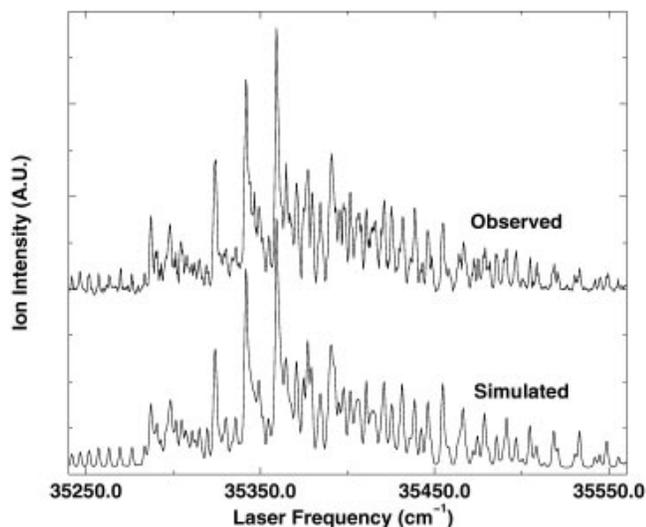
FIG. 3. Upper trace: REMPI spectrum which reflects the internal state distribution of scattered metastable CO molecules. The spectrum is recorded for a gas mixture of 20% CO in Ar and  $\theta_i = 51^\circ$ . Lower trace: Best fitting spectrum using  $T_{\text{rot}} = 293$  K, and an overpopulation of the  $\Omega = 1$  component with a factor of 2.5 relative to the other  $\Omega$  components.
