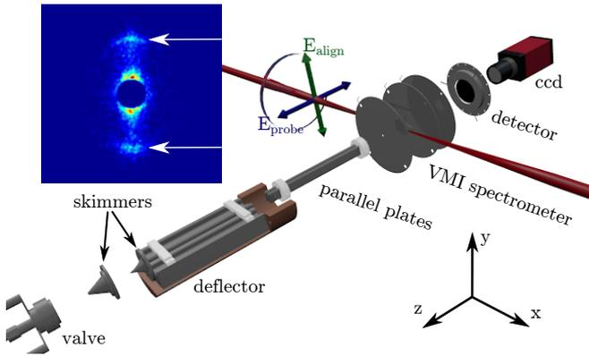
FIG. 1. Schematic of the experimental setup. The inset shows an  $S^+$  ion image recorded when the molecules are aligned along the  $y$ -axis ( $t = 40.6$  ps). The arrows indicate images of the  $S^+ + CO^+$  Coulomb-explosion channel employed to determine the degree of alignment.
