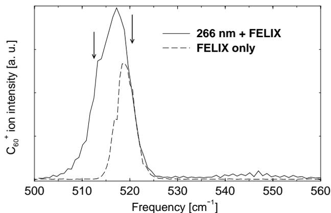
FIG. 3. IR-REMPI spectrum obtained after preexciting  $C_{60}$  with 266 nm radiation to its triplet state (solid line) compared to the IR-REMPI spectrum of  $C_{60}$  as obtained with the IR laser only (dashed line). The arrows indicate the IR laser frequencies that are used to record the TOB distributions shown in Fig. 4.
