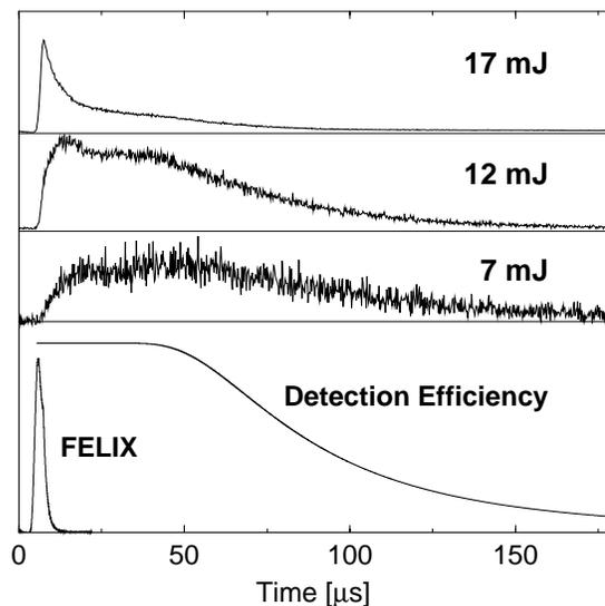
FIG. 2. Time-of-birth (TOB) distributions of  $C_{60}^+$  ions at three different macropulse energies. The envelope of the FELIX micropulses is shown in the lower part together with the time dependence of the experimental detection efficiency.
