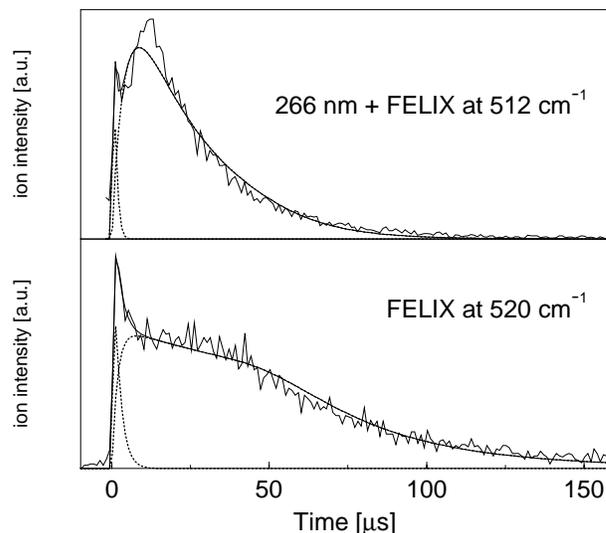
FIG. 4.  $C_{60}^+$  TOB distributions obtained when exciting triplet  $C_{60}$  with FELIX at a frequency of 512  $\text{cm}^{-1}$  (upper part) and when exciting singlet  $C_{60}$  with FELIX at a frequency of 520  $\text{cm}^{-1}$  (lower part). The smooth curves result from fits, each being the sum of two components with the functional form as given in Eq. (2). The dotted curves give the individual components.
