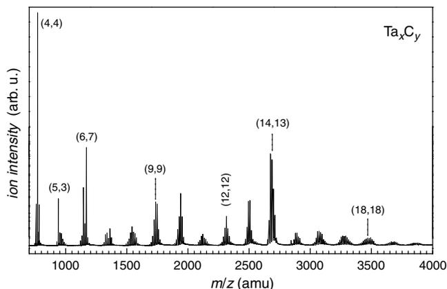
FIG. 3. Mass distribution of  $\text{Ta}_x\text{C}_{y+}$  cluster ions formed via thermionic emission. The mass spectrum has been integrated while FELIX is tuned through the 400–770  $\text{cm}^{-1}$  region.
