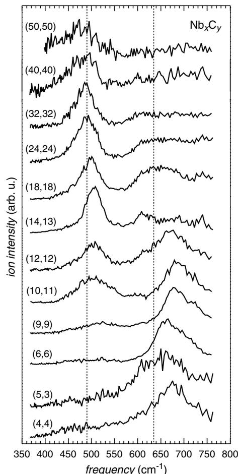
FIG. 2. Infrared spectra for several  $\text{Nb}_x\text{C}_y$  clusters, indicated as (x, y). Except the (5, 3) all clusters may be viewed as parts of a fcc lattice. The two dashed lines indicate the frequencies of optical active surface vibrational modes of fcc NbC (100) measured by EELS [21].
