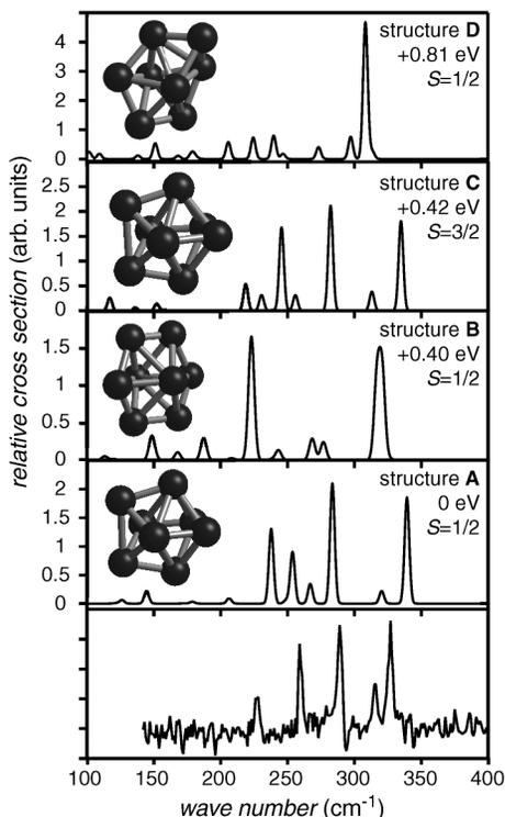
FIG. 4. Comparison of experimental IR spectra for  $V_8^+$  with calculated IR absorption spectra of some isomers. The calculated frequency spectrum is scaled by a constant factor of 0.87, which was obtained by comparison of the experimental dimer vibrational frequency with that calculated with DFT. The spectra are folded with a Gaussian line shape function of  $4 \text{ cm}^{-1}$  width (FWHM).
