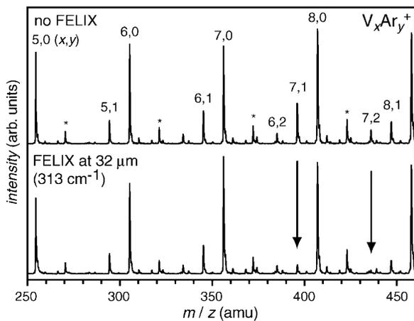
FIG. 2. Part of mass spectra of vanadium cluster cations and their argon adducts. The arrows in the lower mass spectrum show the depleted signals for  $\text{V}_7\text{Ar}^+$  and  $\text{V}_7\text{Ar}_2^+$ , which have an intense resonance around  $313\text{ cm}^{-1}$ . (The asterisks mark oxide contaminations  $\text{V}_n\text{O}^+$ .)
