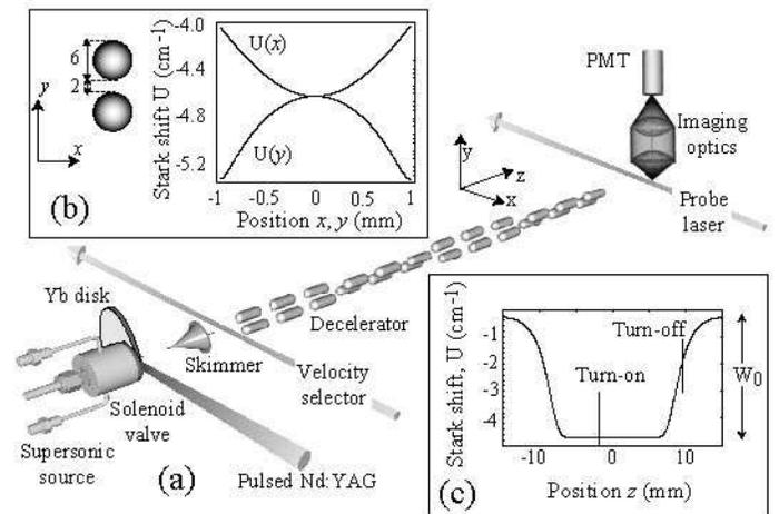
FIG. 1: (a) The beam line. (b) Left: end view of one decelerator stage. Graph: Stark shift of ground state YbF within the stage versus  $x$  and  $y$  for electrode voltages of  $\pm 10$  kV. (c) Same Stark shift versus  $z$ , plotted for one stage.
