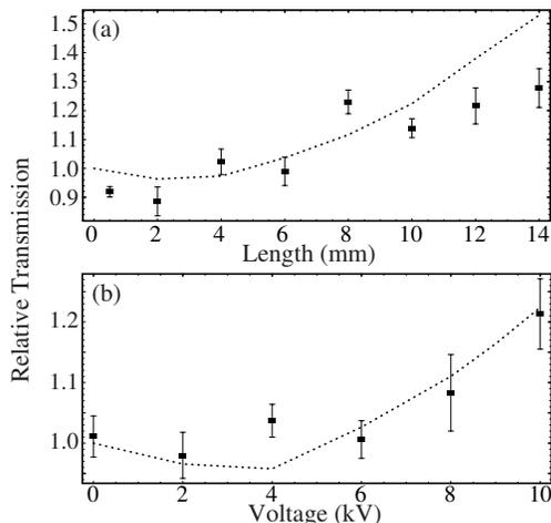
FIG. 5: Normalized decelerator transmission versus (a) effective lens length at a voltage of  $\pm 10$  kV, and (b) electrode voltage for a fixed lens length of 10 mm. Dotted lines: calculation using matrix approach.
