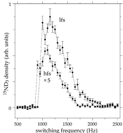
FIG. 3: Density of  $^{15}\text{ND}_3$  molecules in low-field seeking (lfs) and high-field seeking (hfs) levels of the  $|J, K\rangle = |1, 1\rangle$  state at the center of the trap as a function of the switching frequency, after the trap has been on for 72 ms. The signal of the high-field seekers is scaled up by a factor of 5.
