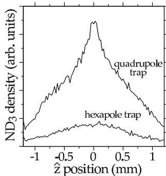
FIG. 6: Density of trapped  $^{15}\text{ND}_3$  molecules as a function of position in the  $z$ -direction for both the quadrupole trap (upper trace) and the hexapole trap (lower trace), after trapping for about 72 ms.
