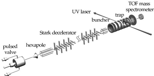
FIG. 5: Experimental setup. A pulsed supersonic beam of  $^{15}\text{ND}_3$  molecules seeded in Xenon exits a cooled valve with a velocity of 280 m/s. Ammonia molecules in the low-field seeking hyperfine levels of the  $|J, K\rangle = |1, 1\rangle$  state are focused into the decelerator by a hexapole, decelerated, and then transversally and longitudinally focused into the trap by a hexapole and buncher, respectively. The molecules are detected in a TOF-mass spectrometer.
