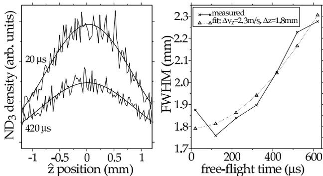
FIG. 8: Determination of the temperature of a packet of  $^{15}\text{ND}_3$  molecules trapped in the hexapole trap. On the left, the profile of a packet is shown  $20 \mu\text{s}$  and  $420 \mu\text{s}$  after the trap is turned off (upper and lower trace, respectively). From a fit to a Gaussian lineshape the FWHM of the distribution is obtained, as shown as a function of free-flight time (solid line with crosses) on the right-hand side of the figure.
