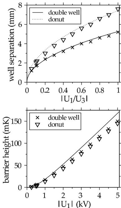
FIG. 4: Well separation as a function of  $|U_1/U_3|$  and barrier height (for  $^{15}\text{ND}_3$ ) as a function of  $|U_1|$  in the ideal double-well (solid line) and donut trap (dotted line). In both graphs the crosses (double-well trap) and triangles (donut trap) show the same quantities obtained from electric field simulations of the actual trap geometry.
