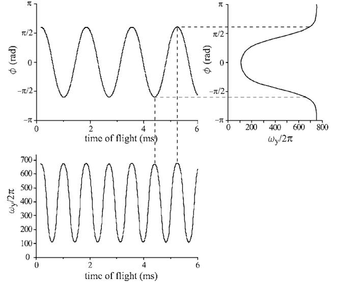
FIG. 5. The temporal dependence of the transverse oscillation frequency  $\omega_y$  can be constructed from the temporal dependence of the phase  $\phi$  in combination with the dependence of  $\omega_y$  on  $\phi$  (Fig. 2).
