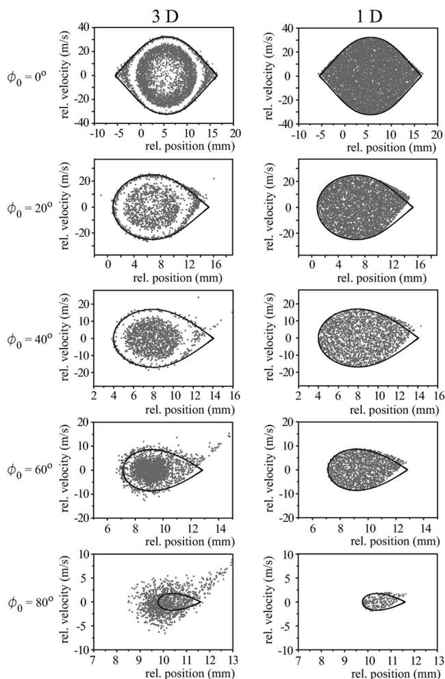
FIG. 3. Longitudinal phase-space distributions of OH ( $X^2\Pi_{3/2}$ ,  $J=3/2$ ,  $M_J\Omega=-9/4$ ) radicals inside the decelerator that result from 1D and 3D trajectory simulations when the Stark decelerator is operated at  $\phi_0=0^\circ$ ,  $20^\circ$ ,  $40^\circ$ ,  $60^\circ$ , and  $80^\circ$ . In all simulations, the molecules spend approximately 8 ms in the decelerator.
