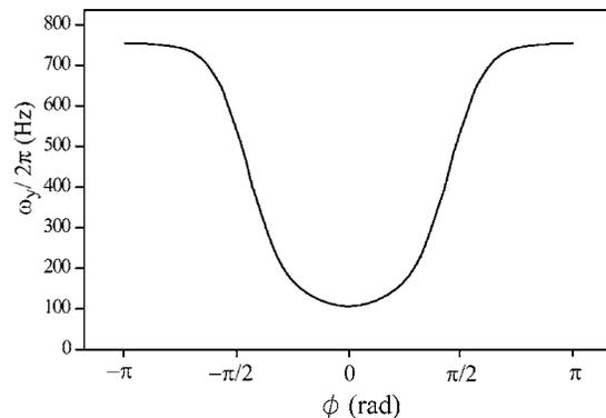
FIG. 2. Natural transverse oscillation frequency  $\omega_y/2\pi$  of the Stark decelerator for an OH ( $X^2\Pi_{3/2}, J=3/2, M_J\Omega=-9/4$ ) radical as a function its phase  $\phi$ .
