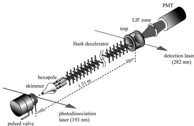
FIG. 9. Scheme of the experimental setup. A pulsed beam of OH radicals is produced via photodissociation of  $\text{HNO}_3$  seeded in Xe. The beam passes through a skimmer, hexapole, and Stark decelerator and is detected via state-selective LIF detection inside the quadrupole trap. The trap is grounded in the present experiments.
