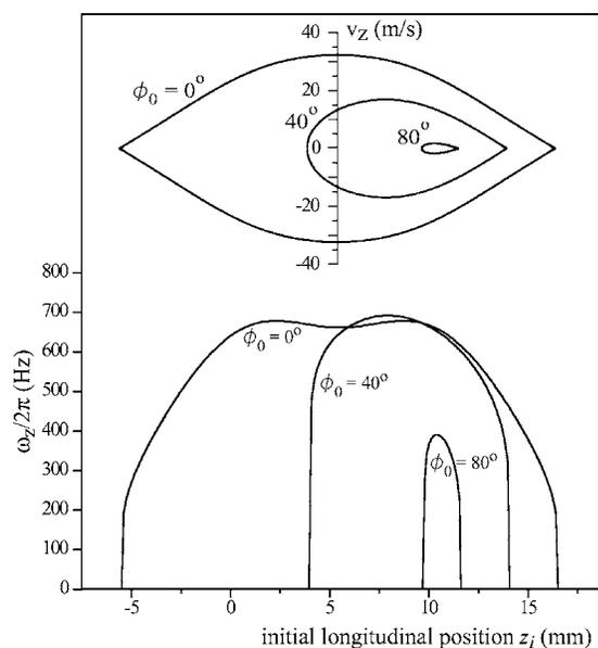
FIG. 1. The natural longitudinal frequencies  $\omega_z/2\pi$  for an OH radical in the  $M_J\Omega=-9/4$  component of the  $X^2\Pi_{3/2}$ ,  $v=0$ ,  $J=3/2$  rotational ground state for the phase angles  $\phi_0=0^\circ$ ,  $40^\circ$ , and  $80^\circ$  as a function of the initial longitudinal position  $z_i$ . For these phase angles, the longitudinal phase-space acceptance diagrams that follow from the 1D model for phase stability are shown in the upper part.
