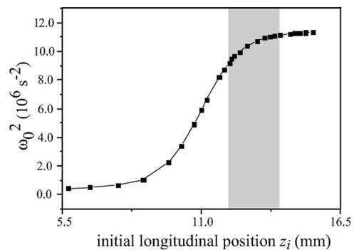
FIG. 7. The time-averaged transverse oscillation frequency  $\omega_0^2$  for an OH ( $X^2\Pi_{3/2}$ ,  $J=3/2$ ,  $M\Omega=-9/4$ ) radical as a function of the initial longitudinal position in the Stark decelerator if the decelerator is operated at  $\phi_0=0^\circ$ . The range in which the decelerator is unstable is indicated by the gray area.
