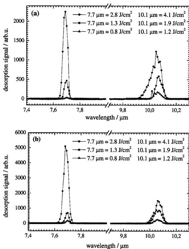
FIG. 4. Desorption spectra of isotopically mixed layers ( $\text{CH}_4:\text{CD}_4 = 50:50$ ) resonantly excited via the  $\nu_4$  bending modes of the isotopes at 7.69 and 10.11  $\mu\text{m}$ . The desorption yield for  $\text{CH}_4$  (a) is monitored on mass 15 and for  $\text{CD}_4$  (b) on mass 20 for different laser energies. Layer thickness and temperature are kept comparable during the experiments; the experimental parameters of FELIX are indicated.
