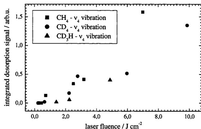
FIG. 2. Dependence of the desorption signal on the laser fluence for multi-layers of  $\text{CH}_4$ ,  $\text{CD}_4$ , and  $\text{CD}_3\text{H}$  condensed on  $\text{NaCl}(100)$  after resonant excitation of the  $\nu_4$  mode at 7.69, 10.11, and 9.75  $\mu\text{m}$ , respectively.
