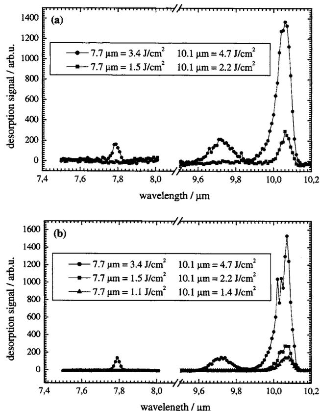
FIG. 6. Desorption spectra of randomly mixed layers of  $\text{CD}_4:\text{CD}_3\text{H} = 50:50$  resonantly excited via the  $\nu_4$  mode of  $\text{CD}_4$  and the  $\nu_2$  and  $\nu_4$  modes of  $\text{CD}_3\text{H}$ . The desorption yield is monitored (a) on mass 16 for  $\text{CD}_4$  and (b) on mass 19 for  $\text{CD}_3\text{H}$ . Different laser-pulse energies are indicated.
