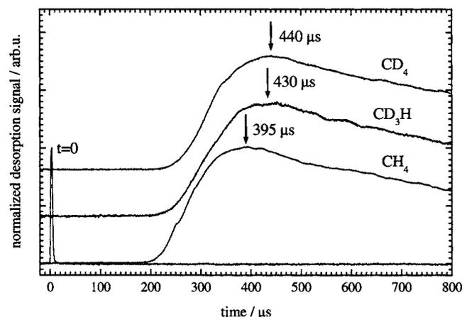
FIG. 3. Time-of-flight spectra for the desorption of  $\text{CH}_4$ ,  $\text{CD}_4$ , and  $\text{CD}_3\text{H}$  recorded at the resonance frequencies of the  $\nu_4$  mode. The maxima of the flight-time distribution are indicated for each time-of-flight spectrum in the figure. The spectra are offset for clarity.
