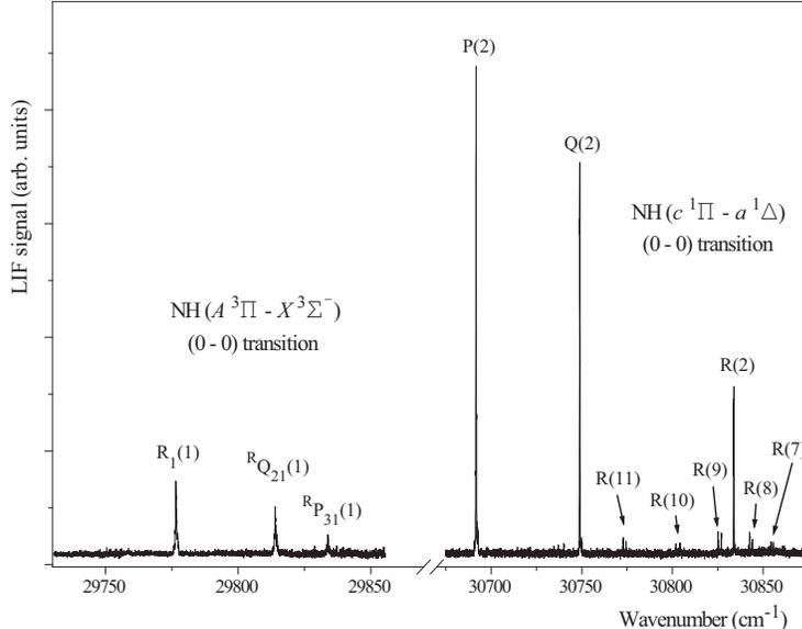
Fig. 1. Fluorescence excitation spectrum of the  $A^3\Pi, v = 0 \leftarrow X^3\Sigma^-, v = 0$  band and the  $c^1\Pi, v = 0 \leftarrow a^1\Delta, v = 0$  band of NH in the pulsed molecular beam. The lines are labelled using standard spectroscopic nomenclature.
