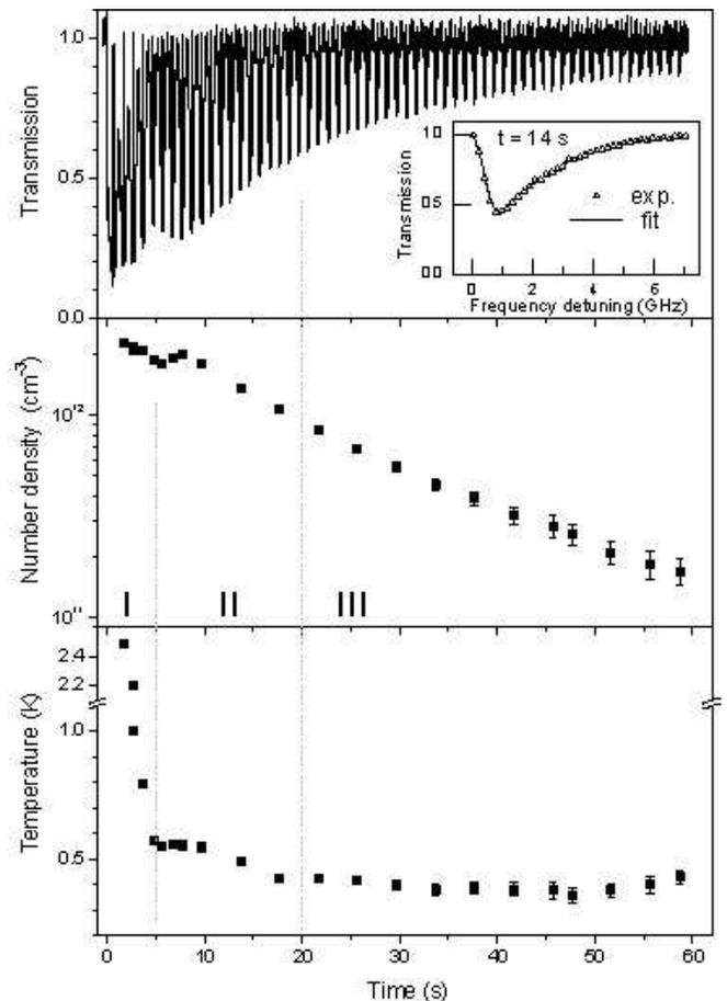
FIG. 2: Transmission through a sample of Cr atoms in the buffer gas cell (top graph). The probe laser frequency is scanned repeatedly over the atomic transition with a repetition rate of  $1$  Hz. The inset shows a typical absorption profile (triangles) after  $\sim 14$  s, together with a simulation (dotted line). The other two graphs show the evolution of the particle density (middle) and temperature (bottom graph) of the trapped atom ensemble over time.
