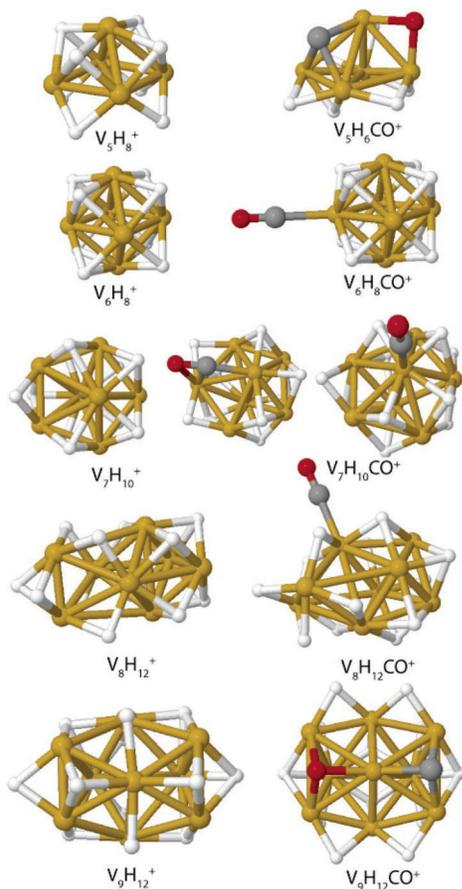
**Figure 3.** Geometric structures of isomers of saturated  $V_nH_m^+$  (left) and  $V_nH_mCO^+$  complexes (right) for  $n = 5-9$  selected on the basis of the comparison of experimental and calculated IR spectra.
