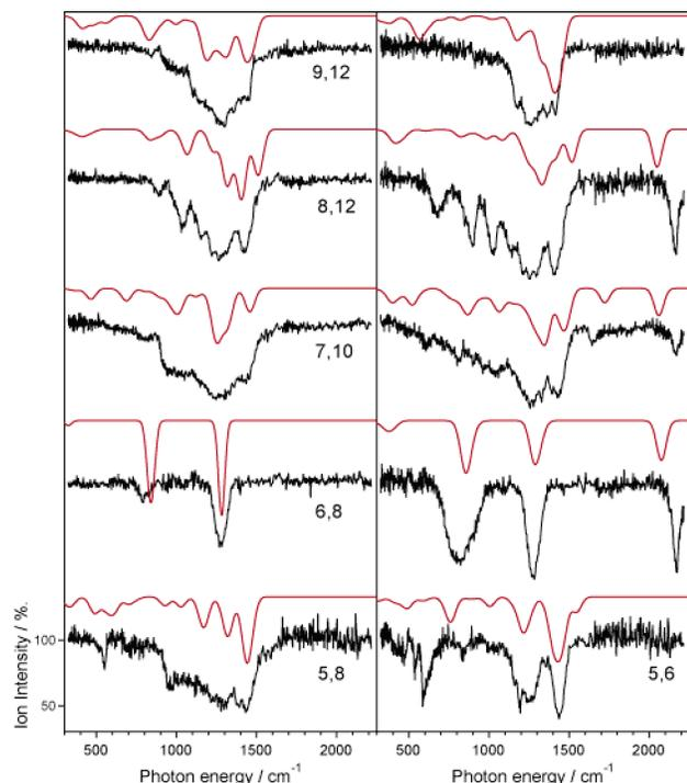
**Figure 2.** IR-MPD spectra (black) of fully saturated  $V_nH_m^+$  (left panel) and the corresponding  $V_nH_mCO^+$  complexes for  $n = 5-9$  (right panel, bottom to top). Values of  $n$  and  $m$  for the fully saturated clusters are denoted as  $n,m$  in the graph. The spectra depicted in red are calculated IR spectra for the structures shown in Figure 3. The calculated spectrum of  $V_7H_{10}CO^+$  is a linear combination of the two isomers depicted.
