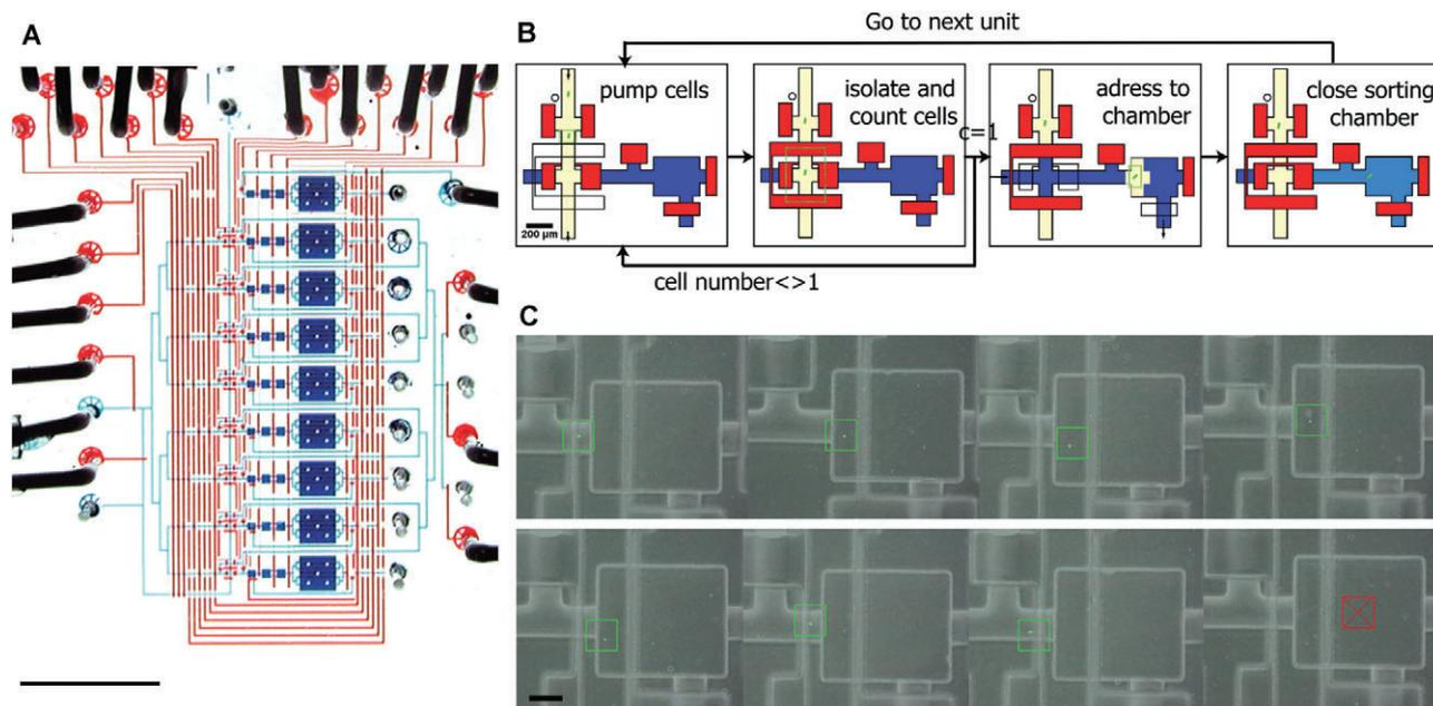
**Fig. 1.** Photograph of a single-cell isolation and genome amplification chip capable of processing nine samples in parallel (eight cells, one positive control).
