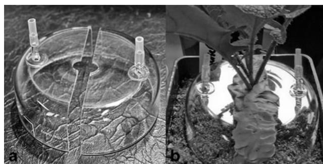
**Fig. 2** Cuvette used for dynamic headspace collections from plant roots. **a** the cuvette which consists of two parts with an air in- and outlet, respectively. **b** cuvette fitted together and tightened with a rubber-based sealant
