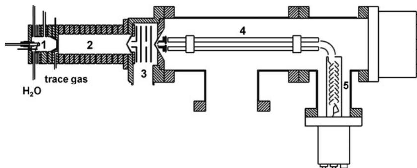
**Fig. 1** Schematic representation of a typical PTR-MS. The instrument consists of an ion source (1) in which  $H_3O^+$  primary ions are produced, a drift tube (2), where the trace gases from samples are ionized by the proton-transfer reaction with  $H_3O^+$  ions, a collisional dissociation
