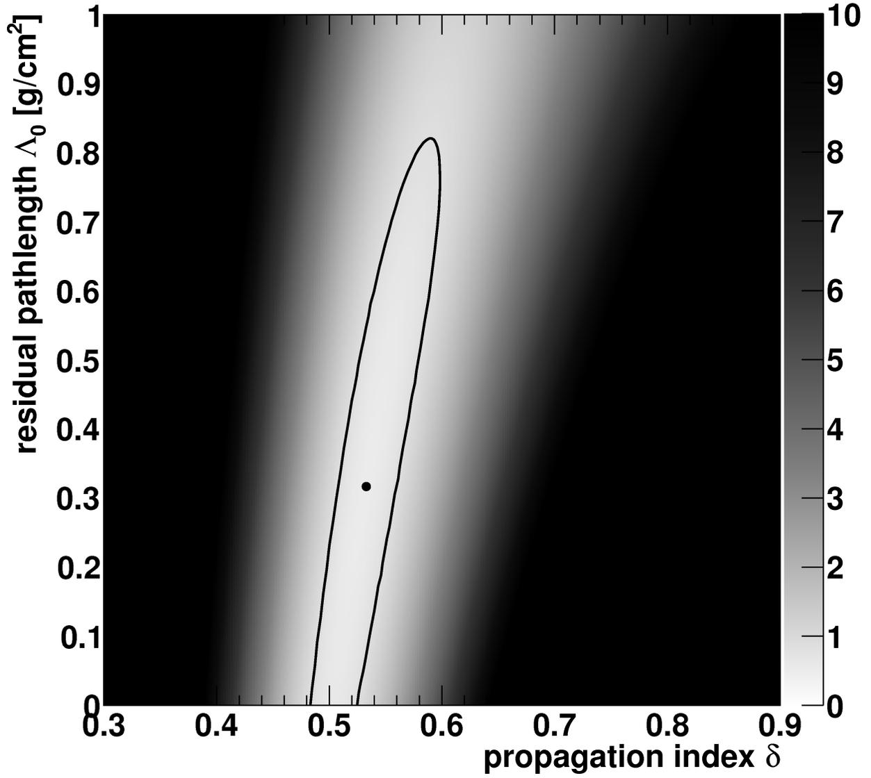
Fig. 3.—  $\chi^2$  map in the parameter space of  $\delta$  vs.  $\Lambda_0$  for the Leaky-Box model fit to TRACER data. The best fit values are marked at  $(\delta, \Lambda_0) = (0.53 \pm 0.06, 0.31^{+0.55}_{-0.31} \text{ g cm}^{-2})$  and the  $1\sigma$  contour is indicated.
