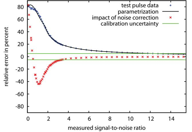
Figure 4: Relative uncertainty of the true pulse height ( $\Delta A_{\text{true}}/A_{\text{true}}$ , x), in each bin of the measured signal-to-noise ratio  $A_{\text{meas}}$ . This is compared with the error one would make, if the measured pulse amplitude would not be corrected for the noise influence ( $(A_{\text{true}} - A_{\text{meas}})/A_{\text{true}}$ , +), and with the calibration uncertainty due to environmental effects (horizontal lines).
