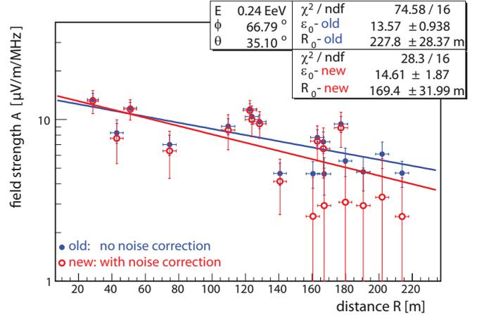
Figure 5: Example lateral distribution from a typical selection with and without correction of the noise influence.
