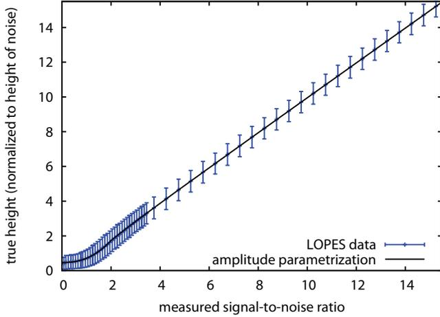
Figure 3: Relation between the true signal height  $A_{\text{true}}$  and the measured signal-to-noise ratio  $A_{\text{meas}}$ . The error bars correspond to the standard deviations of the binned data, i.e.  $\Delta A_{\text{true}}$ , and not the uncertainty of the plotted mean.
