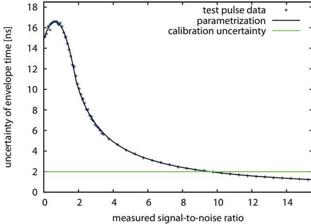
Figure 6: Average deviation between the measured time of the envelope maximum after adding noise, and the original time before adding noise, and the time calibration uncertainty as reference.
