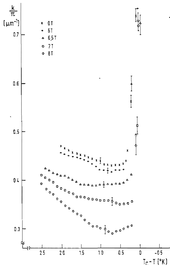
FIG. 3. Temperature dependence of the inverse pitch at different applied magnetic fields.
