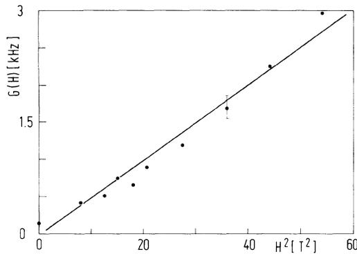
FIG. 4. Magnetic-field dependence of the gap  $G(H)$ , separating the optic and acoustic phason modes at  $q=0$ ,  $T_c - T = 3$  K. The difference between the normalized optic and acoustic phason relaxation rates was multiplied by the mean value of 1.5 kHz for both relaxation rates at zero field (see text) to obtain  $G(H)$ .
