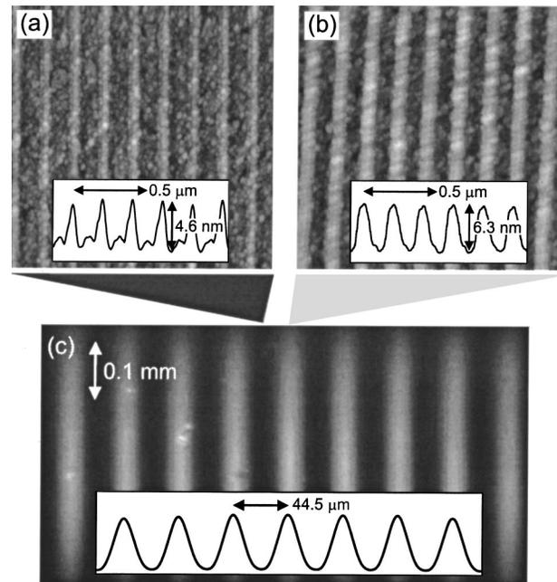
FIG. 2. Superimposed depositions at the  $J=3 \rightarrow 3$  and  $J=3 \rightarrow 4$  transitions. (a), (b) AFM scans at the nearly out-of-phase (a) and nearly in-phase (b) regions. Insets in (a), (b): Profiles averaged over  $2 \mu\text{m}$  along the lines. (c) Optical microscope image obtained in transmission. The sample was placed at  $45^\circ$  between a polarizer and a crossed analyzer. Inset in (c): Intensity profile averaged over  $0.3$  mm along the lines.
