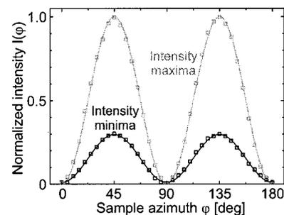
FIG. 3. Analysis of the beating pattern in a transmission optical microscope. The sample was placed between a polarizer and a crossed analyzer. Light intensity  $I(\varphi)$  at the in-phase (intensity maxima) and out-of-phase (intensity minima) regions as a function of the azimuth  $\varphi$  of the sample. Squares—data points, lines— $I(\varphi) \propto \sin^2(2\varphi)$ .
