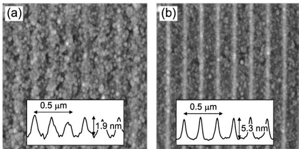
FIG. 1. AFM scans of laser-focused Cr nanolines on an ITO substrate. Depositions carried out at the  $J=3 \rightarrow 3$  (a) and  $J=3 \rightarrow 4$  (b) transitions. Insets: Profiles averaged over  $2 \mu\text{m}$  along the lines.
