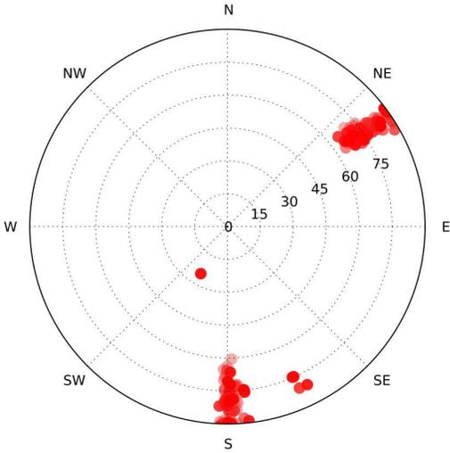
Figure 3: Example of pulse arrival directions as calculated from trigger arrival times. The center represents the zenith; the outer edge corresponds to the horizon. Shown are two fixed interference sources and one pulse from a high elevation that would pass the trigger conditions.
