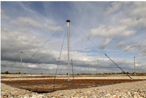
Figure 2: Photograph of a LOFAR droop-dipole low-band antenna (LBA).
