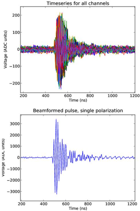
Figure 4: Top: time-series radio signal for all channels individually (superimposed). Bottom: the beam-formed signal, in the same voltage units. Note the much larger pulse height as well as a larger signal-to-noise ratio in the beam-formed signal.
