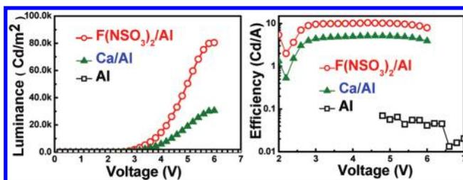
**Figure 1.** (a)  $L$ - $V$  and (b) current efficiency- $vs$ - $V$  characteristics of PLEDs with the following device structures: ITO/PEDOT:PSS/F8BT/F(NSO<sub>3</sub>)<sub>2</sub>/Al (red ○); ITO/PEDOT:PSS/F8BT/Ca/Al (green ▲); ITO/PEDOT:PSS/F8BT/Al (black □).
