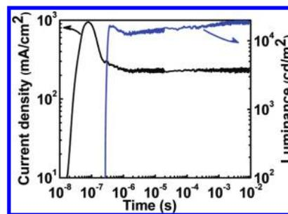
**Figure 2.** Brightness (blue line) and current density (black line) dynamics of ITO/PEDOT:PSS/F8BT/F(NSO<sub>3</sub>)<sub>2</sub>(7 nm)/Al device using rectangular voltage pulses of 4.9 V at a frequency of 1 Hz.
