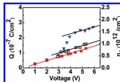
**Figure 3.** Capacitive charge ( $Q$ ) and charge density ( $n_c$ ) calculated (line,  $\epsilon = 3$ ) and measured for an ITO/PEDOT:PSS/F8BT/Ca/Al device (red ●) as well as the sum of displacement charge and capacitive charge from ITO/PEDOT:PSS/F8BT/F(NSO<sub>3</sub>)<sub>2</sub>/Al with a 7 nm (black □) or 12 nm (blue ▼) F(NSO<sub>3</sub>)<sub>2</sub> layer. Thin black lines are guides for the eye.
