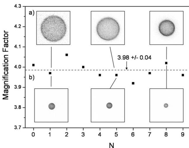
FIG. 5. Insets in (a) show  $\text{NO}^+$  images obtained for individual rotational states of  $\text{NO}(\tilde{A}, v' = 0, N)$  with the magnification lens at 1200 V, and in (b) with the magnification lens at 0 V. Also shown are the measured magnification values for each separate  $N$  state.
