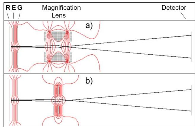
FIG. 1. (Color online) [SIMION software (Ref. 14)] (a) Potential fields for the present design with a 1300 V repeller, 1076 V extractor, and 1142 V magnification lens (center lens in the figure). (b) Potential fields for the standard 3-plate Einzel lens with 1300 V repeller, 1080 V extractor, and 1256 V on the center plate of the Einzel lens.
