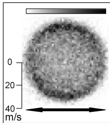
FIG. 3.  $\text{O}^+$  image from a beam of cold  $\text{O}(\text{}^3\text{P}_2)$  atoms formed in a discharge and ionized by (2 + 1) REMPI at 226 nm. Darker areas correspond to higher signal. The arrow marks the direction of the laser polarization. Recoil due to the REMPI process is maximal in the direction perpendicular to the laser polarization and characterized by  $\beta = -0.2$ . Note that the CCD pixel resolution exceeds the imaging detector resolution in this image.
