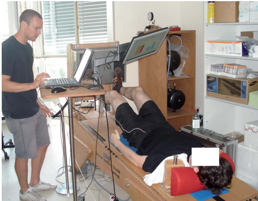
Figure 3. Countermeasure exercise training. Both the resistance exercise only (RE) and resistance exercise with whole-body vibration (RVE) groups performed their exercises on the specially designed Galileo Space exercise device. Subjects performed all exercises in the head-down tilt position and were positioned on a moveable platform with shoulder pads and hand grips preventing downward movement and permitting application of force via the platform. A pneumatic system generated the force, applied through the moveable platform, against which the subject needed to resist and move (via the shoulder pads and hand grips). The feet were positioned on either side of a platform which was set to vibrate during high-load resistive exercises in the RVE-group. Subjects were given visual feedback of their actual and target position in the exercise via a monitor placed in the subjects' field of view. As the force output was dictated by the exercise device, the feedback focused on ensuring the subjects performing the exercise in the desired range of motion and at the desired speed. During the heel raises the sport scientist monitored the range of movement and encouraged the subject to go to the end of range in each direction. Here the subject is performing squats with the knee and hip musculature.
