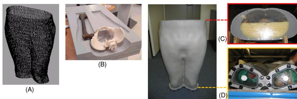
**Figure 1.** Development of the anatomically shaped model of the lower body. (A) The scaled contour of the body model; (B) within the model, a cavity was created for a pelvis and two femurs; (C) at the proximal side, the model was semi-permanently closed; (D) at the distal side, two removable Lucite plates containing air valves were incorporated.
