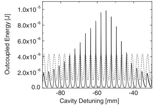
FIG. 2. Detuning curve is shown by the solid line. The initial cavity length is 7.275 m. Dotted curve presents  $\cos(2\delta Lk_z)$  dependence where  $k_z = \sqrt{(2\pi f^-/c)^2 - (\pi/g)^2}$ , where  $g$  is the waveguide gap.
