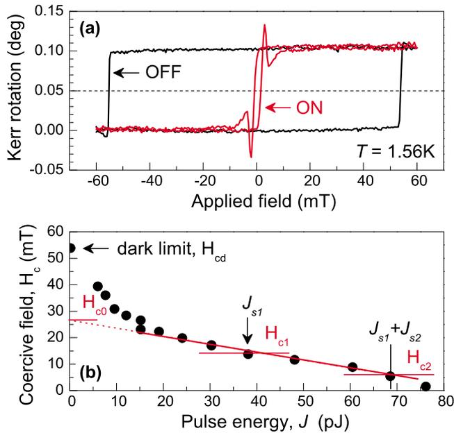
FIG. 2. (Color online) (a) MOKE measurements of magnetic hysteresis of the (Ga,Mn)As film measured with the pulse picker off and on (with  $f=100$  Hz and  $J=76$  pJ). (b) The measured coercive field as a function of pulse energy  $J$ . The vertical arrow indicates the pulse energy  $J_s$  used to measure dynamics of the PCE in Fig. 4.
