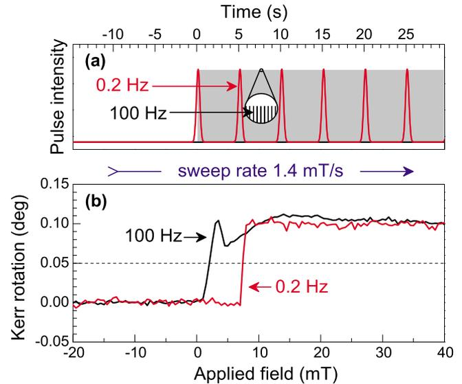
FIG. 3. (Color online) (a) Schematic representation of pulse trains with repetition rate of 100 and 0.2 Hz ( $J=75$  pJ). (b) Magnetic switching observed for repetition rate of 100 and 0.2 Hz. The sweep rate of the magnetic field is 1.4 mT/s. At low repetition rates, switching is delayed until a pulse arrives.
