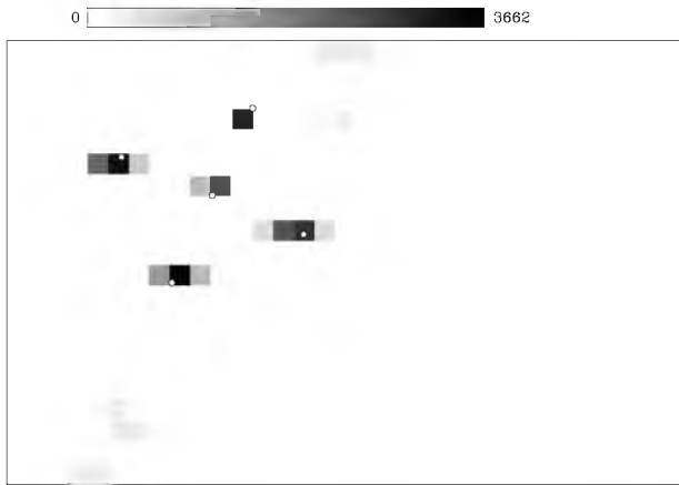
Fig. 9. Negative image of the 5 pinhole pattern. The five circles which represent the predicted pattern on the detector.
