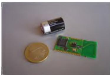
Figure 1: Chess MyriaNode 2.4 Ghz wireless sensor node
