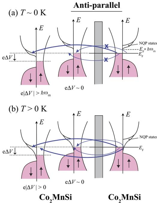
FIG. 4: (Color online) Schematic representation of an electron tunneling process at  $\Delta V \approx 0$  and at finite bias voltage in a  $\text{Co}_2\text{MnSi}/\text{Al-O}/\text{Co}_2\text{MnSi}$  magnetic tunnel junction. At  $T \approx 0\text{K}$  (a), NQP states vanish at  $E_F$ , while for  $T > 0$  (b) (see text) NQP states extends across  $E_F$  and an additional tunneling channel opens.
