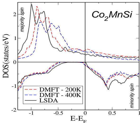
FIG. 1: (Color online) Spin resolved density of states of the  $\text{Co}_2\text{MnSi}$  full-Heusler alloy obtained by LSDA and LSDA+DMFT. The LSDA+DMFT results are obtained for  $U=3\text{eV}$  and  $J=0.9\text{eV}$  (in both Co and Mn), and different temperatures.
