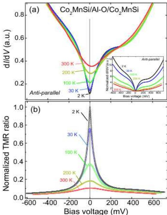
FIG. 2: (Color online) (a) Tunnel conductance for the  $\text{Co}_2\text{MnSi}/\text{Al-O}/\text{Co}_2\text{MnSi}$  anti-parallel magnetic tunnel junction and (b) TMR ratio (normalized to  $T = 2\text{K}$ ,  $V = 0$ ), as a function of voltage for different temperatures. The inset of panel (a) shows the conductance normalized to zero bias voltage.
