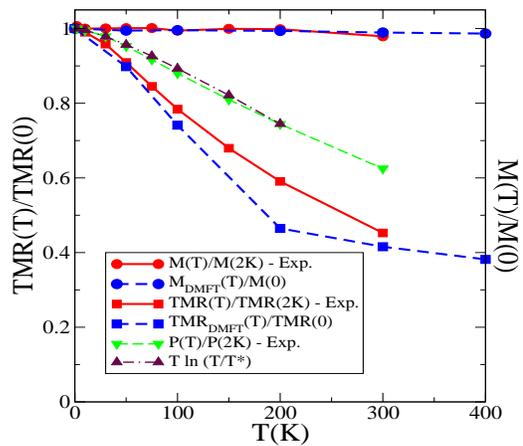
FIG. 3: (Color online) Comparison of the TMR ratio and magnetisation ( $M$ ) as a function of temperature for a  $\text{FeCo}/\text{Al-O}/\text{Co}_2\text{MnSi}$  tunnel junction as obtained from experimental data and from LSDA+DMFT. Triangle-down/up represents the measured polarization and the fit to the analytic expression  $1 - P(T)/P(0) \propto T \ln T/T^*$  [18].
