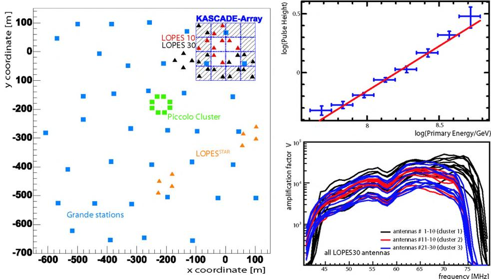
**Figure 1.** Left: Sketch of the LOPES set-up at the KASCADE-Grande experiment. Upper right: Average radio pulse height of the detected events versus the primary particle energy as reconstructed by KASCADE-Grande. Lower right: Frequency dependent amplification factors for all 30 antennas obtained by the amplitude calibration.
