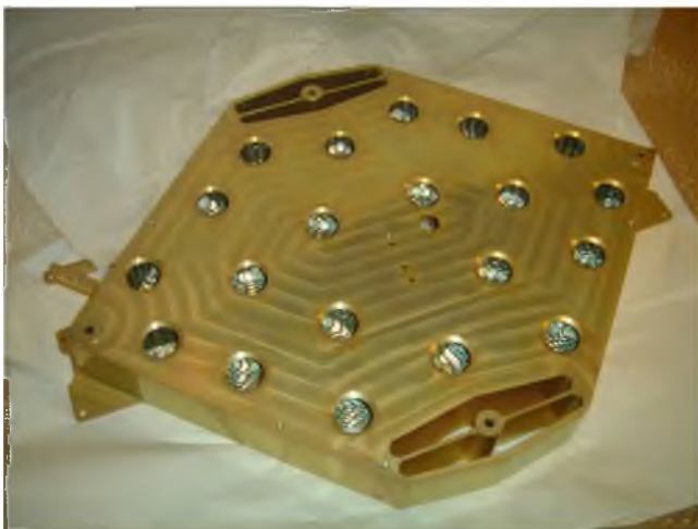
Figure 4. Balance Arm using the ASTRON extreme light-weighting technique. Large internal volumes (pockets) are created by milling through small entrance holes. The weight of the 540 x 400 x 57 mm aluminium balance arm is 2kg, which corresponds to lightweighting percentage of 90%. Internal ribs in the pockets improve the overall stiffness.
